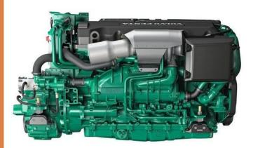
The new D12 is a 12-liter, in-line cylinder power unit with 4 valves per cyl-inder designed to offer high performance for smaller commercial vessels. The en-gine comes in two versions for commercial applications: the D12-650 develop-ing 650 hp (478 kW) and the D12-615 with an output of 615 hp (453 kW). Both versions have the same
